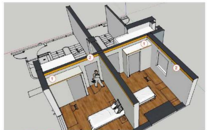
View 3 - typical room to first floor rear elevation 1 - pod ensuite inserted into existing room 2 - Existing cornice
