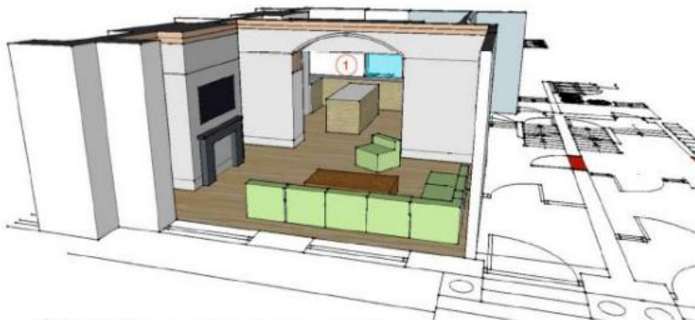
View 4 - typical ground floor lounge/kitchen 1 - form new opening in existing archway (as house 6 - see photo)
