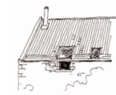
Conservation Rooflight – this is well suited to older buildings due to its low profile within the roof plane
