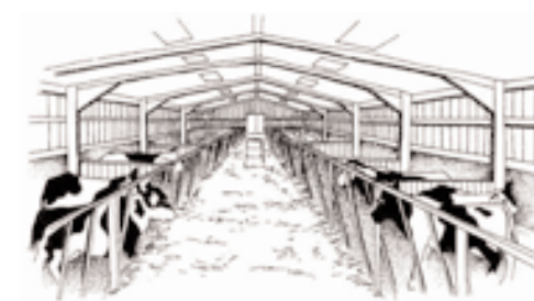
Interior of a typical modern farm building showing shallow roof pitch and portal frame construction.
