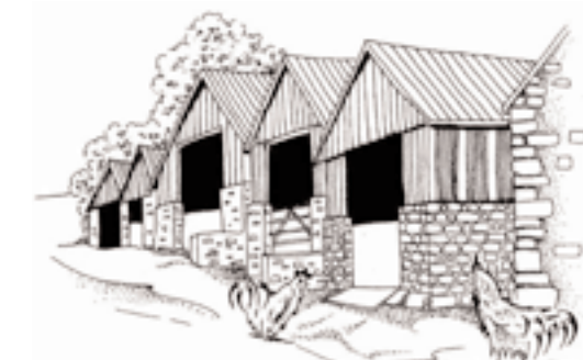
A stepped construction on a sloping site helps break up an otherwise unbroken roof line.
