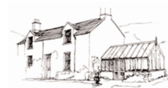
Dwarf walls for a conservatory should be built in the same material as the main house
