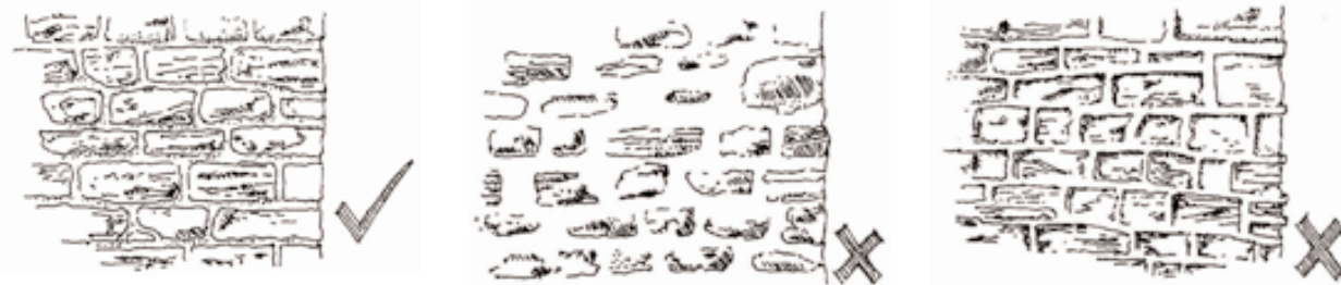
Mortar slightly recessed allows the stones to 'read'
