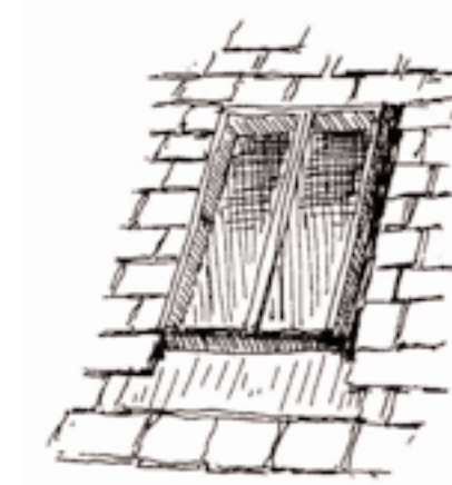
Conservation Rooflight – this is well suited to older buildings due to its low profile within the roof plane
