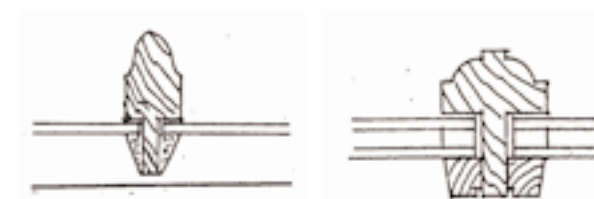
Left, traditional single glazing detail and right, acceptable solution for double glazing
