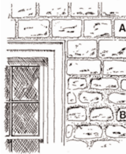
A Good pointing finished just behind stone face B Bad pointing smeared over the face of stones
