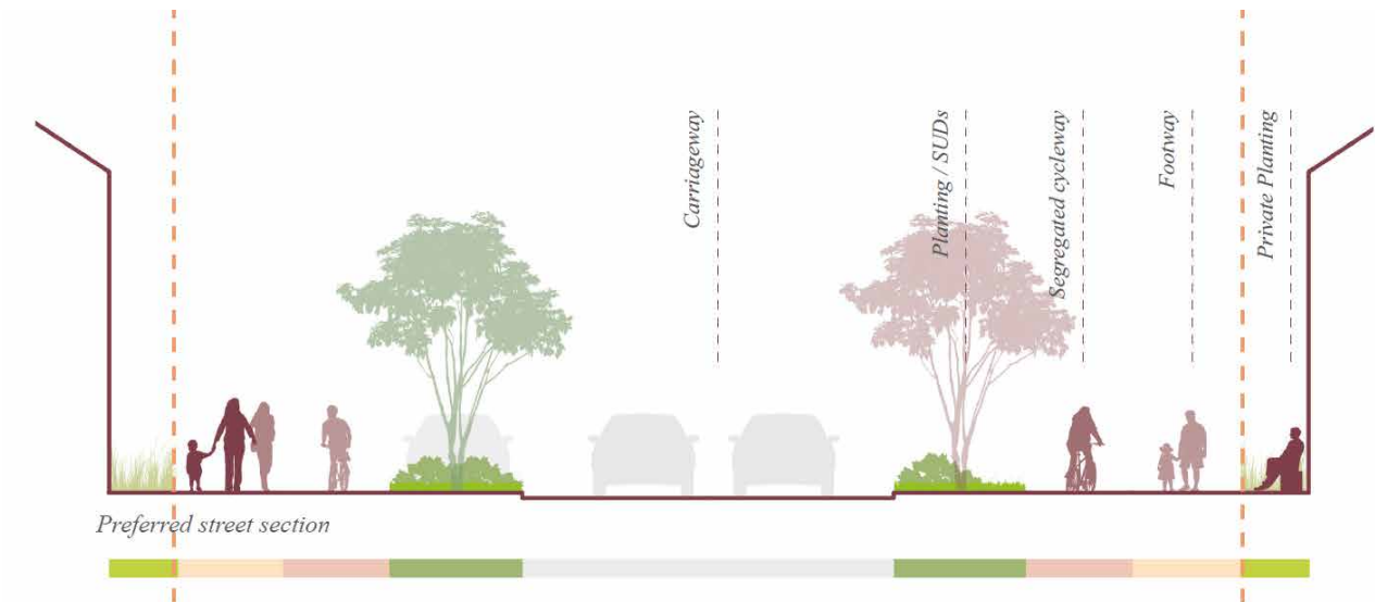
Figures 23: Preferred Street Section (Source Arup)
