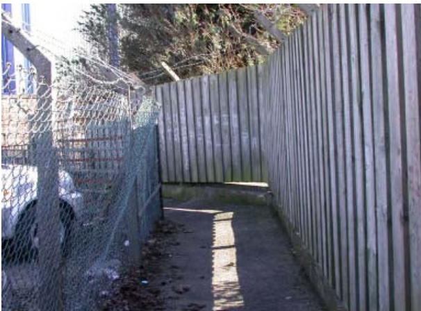
Pedestrian routes should be attractive and safe to use. This example has poor through-visibility and does not invite use.
