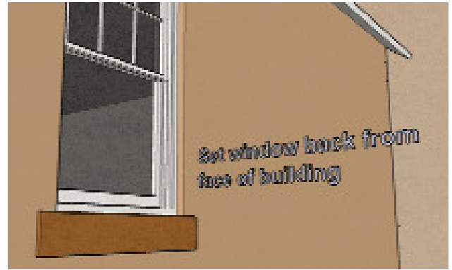
Fig 64. Windows set back from the facade protect timber from the elements and add can depth and visual interest to the elevation.
