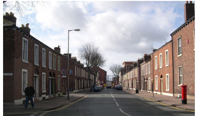
Fig 75. In terraces, a limited field of vision for passing pedestrians results in greater privacy to residents than if houses were set further back from the pavement edge.
