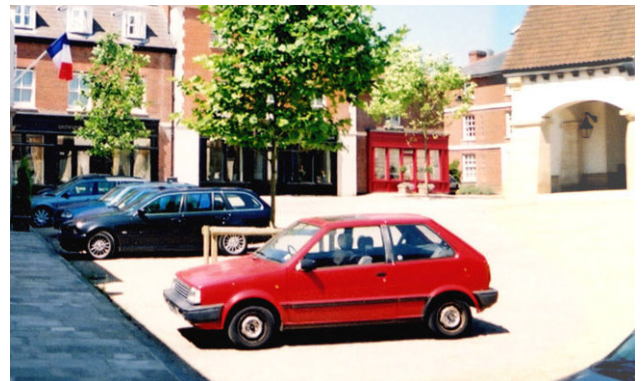
Fig 14. Unmarked parking bays - When not occupied by vehicles the space takes on a civic appearance, rather than appearing as merely an empty car park.
