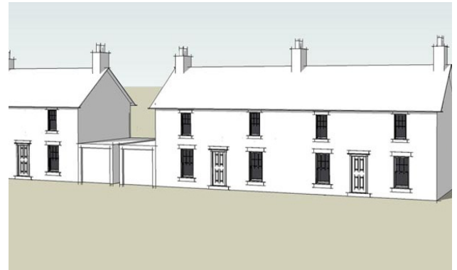
Fig 87. A street of semi detached houses with garages between. It is important to avoid creating a terracing effect by incremental extensions.
