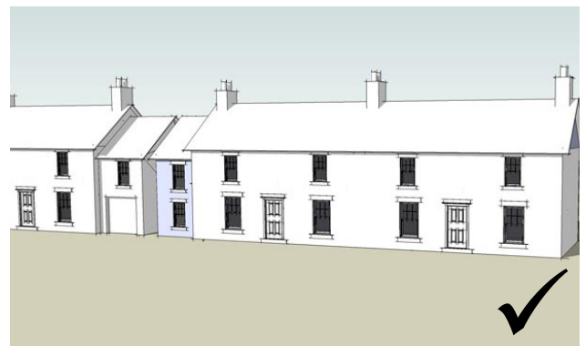
Fig 89. A preferred approach to extending would be to create subordinate extensions that maintained the primacy of the original houses.
