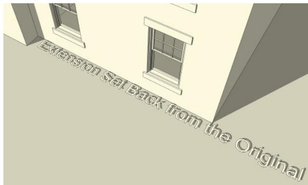
Fig 87. An extension should usually be set back from the original dwelling - 500mm is suggested.
