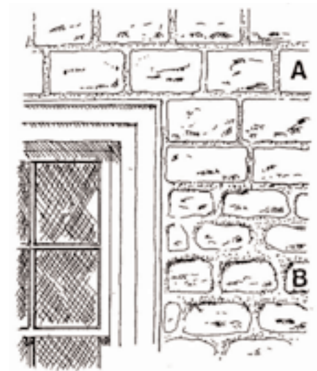
A Good pointing finished just behind stone face B Bad pointing smeared over the face of stones
