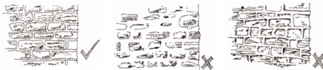
Mortar slightly recessed allows the stones to 'read'
