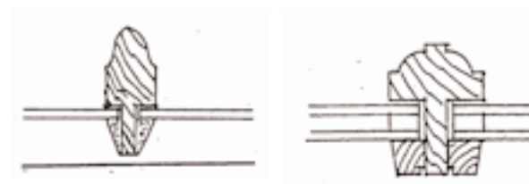
Left, traditional single glazing detail and right, acceptable solution for double glazing
