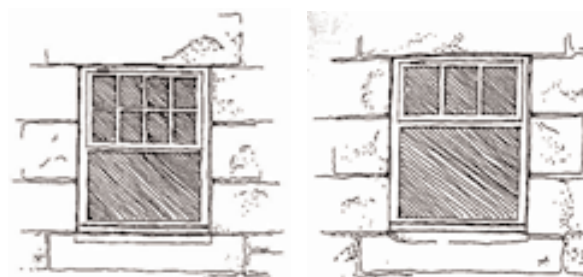
Above, traditional single glazing detail and below, an acceptable solution for double glazing
