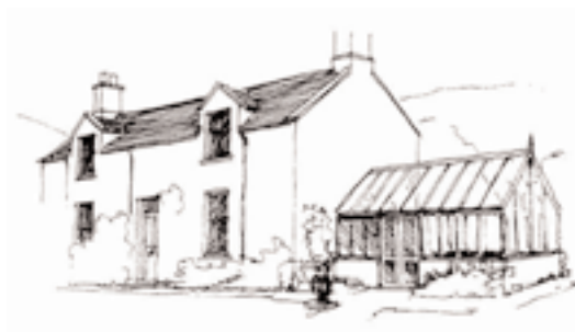
Dwarf walls for a conservatory should be built in the same material as the main house
