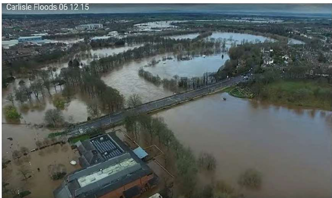
Figure 7 Upstream from the Sands. Note quiet water upstream and angry water downstream. The bridge is clearly acting as a dam restricting conveyance
