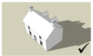
Fig 87. Where possible dormer windows and veluxes should be located on rear elevations.
