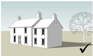
Fig 86. An extension should be secondary in scale and massing to the original dwelling house.
