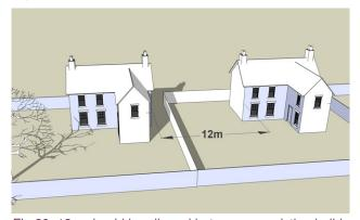
Fig 80. 12m should be allowed between an existing building and any blank gable or wall to any new building.
